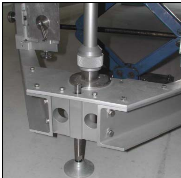
The template clamp, fine adjustment system, precision alignment line and levelling feet used to precisely position the templates so that they are vertical and in the section planes.
