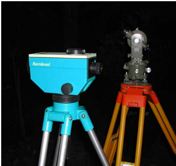
Figure 8.3.8 a - Surveyor's level and theodolite
