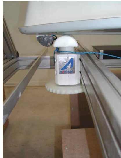
470 Jig with a hull on top (left) and the modular framing and levelling screws detail (right)
